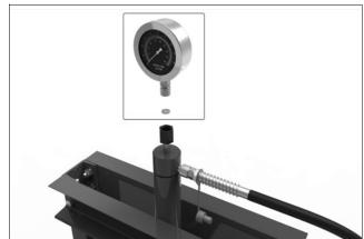
7. Making sure the gauge faces the front of the press, using two spanners, tighten the gauge nuts as shown.
