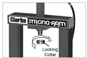
4. Using two spanners, unscrew the transportation cap from the top of the press cylinder as shown.
